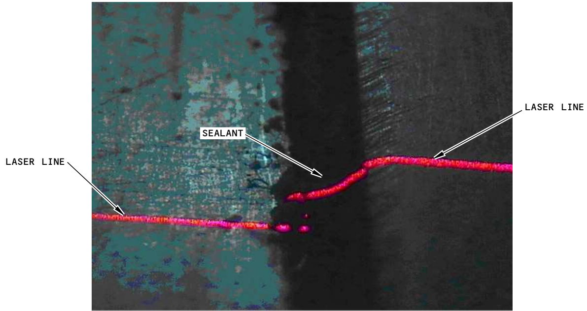
THIS PHOTOGRAPH SHOWS THE EFFECT ON THE LASER LINE FROM SEALANT AT THE EDGE OF THE LAP.
